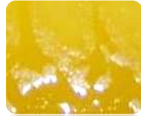
Stearin crystal formation
